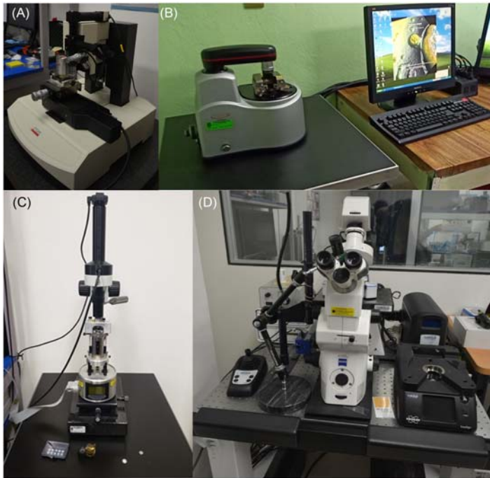
Figure 9.8 Examples of instruments for obtaining micro and nanomechanical properties used in food science, (A) microindenter (TTX-NHT, CSM Instruments, Switzerland), with a diamond Berkovich tip (pyramidal geometric), (B) basic atomic force microscope (Dilnova, Veeco, USA), (C) classic model of an atomic force microscope (Multimode, Veeco, USA), (D) BioAFM (Bioscope Catalyst, Bruker, USA).
